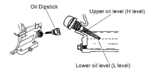
**IMPORTANT:** The Oil Shortage Alarm System is designed to avoid damage of the engine due to shortage of oil in the crankcase. The system will automatically shut down the engine just before the crankcase oil level drops down to the minimum line of safety.
