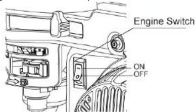
**NOTE:** Turn the engine switch to the OFF position immediately to shut down the engine in an emergency.
